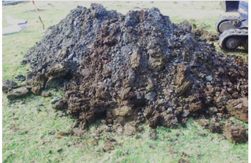
Figure 38: Sediments sampled at Friog. The excavated material shows a mixture of orange-brown sand and grey clay.
