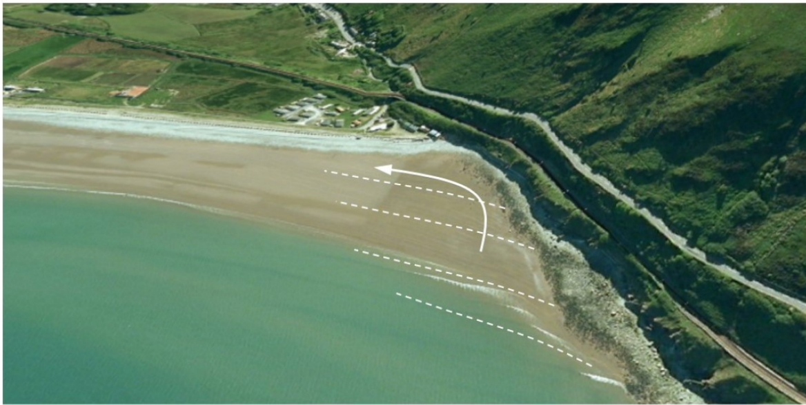
Figure 15: Approach of waves at Friog corner, and redirection of the water mass along the spit.
