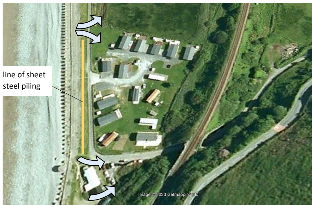
Figure 25: Location of the line of sheet steel piling, and observed water flows at the northern and southern ends.
